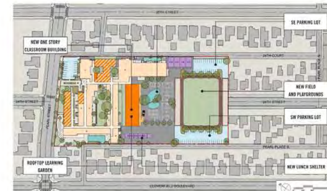
GROUP 1 PROJECTS Could include a one story classroom building with rooftop learning garden, relocated field and playgrounds, new parking lots
